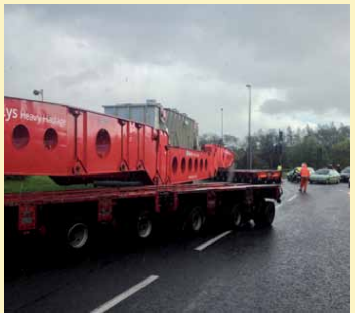
The huge vehicle is 100m long and 5m wide and took up two lanes of the motorway while it crawled to its final destination at walking pace.
