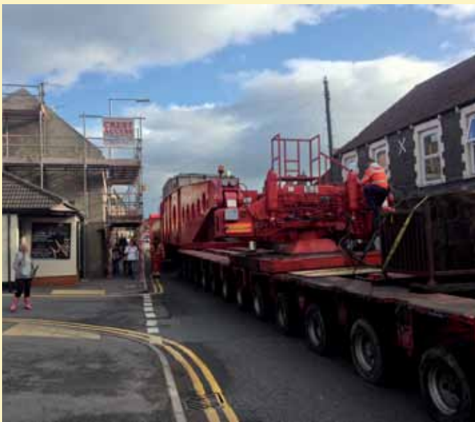
An enormous transformer was carried from Didcot power station, but was transported at just 4mph as it weighed 640 tonnes.
